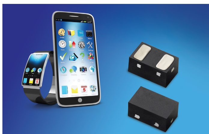
Figure 4: Low-capacitance bidirectional discrete TVS diode arrays, including the SP3522 Series, provide symmetrical ESD protection for high-speed data lines when AC signals are present. They are also designed for consumer electronics such as fitness bands, smartwatches, smartphones, tablets and eReaders.
