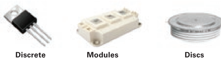
Figure 5: Power Semiconductor Device Packaging
