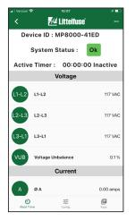
Get Real-time system status readings for voltage, current, power, time-delay. It's a volt meter, amp meter, power meter, and diagnostic tool in the palm of your hand.
