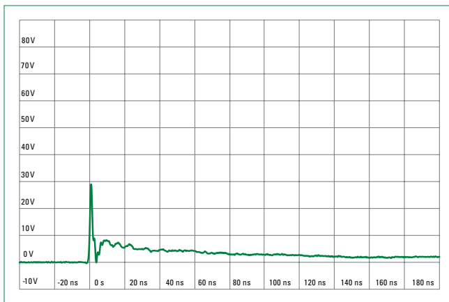
IEC 61000-4-2 +8 kV Contact ESD Clamping Voltage
