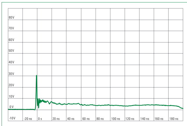
IEC 61000-4-2 +8 kV Contact ESD Clamping Voltage
