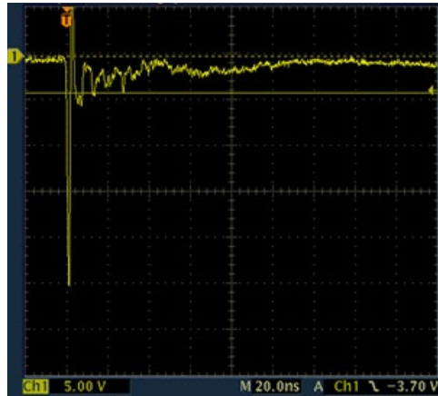
SP1124 IEC 61000 -4-2 -8 kV Contact ESD Clamping Voltage
