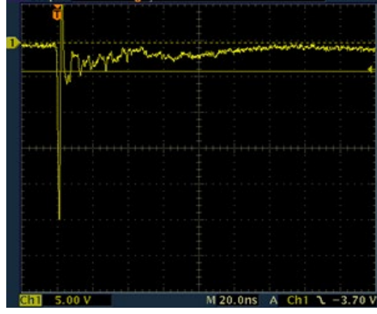
SP1105S IEC 61000 -4-2 -8 kV Contact ESD Clamping Voltage
