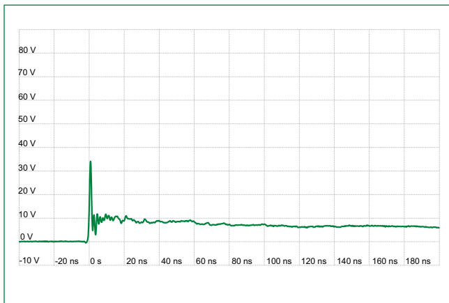
IEC 61000-4-2 +8 kV Contact ESD Clamping Voltage
