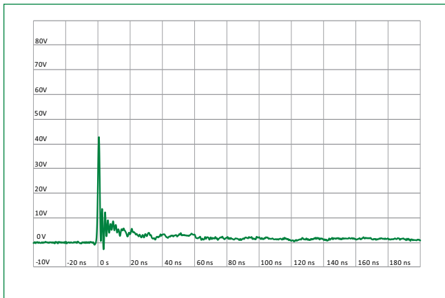
IEC 61000-4-2 +8 kV Contact ESD Clamping Voltage
