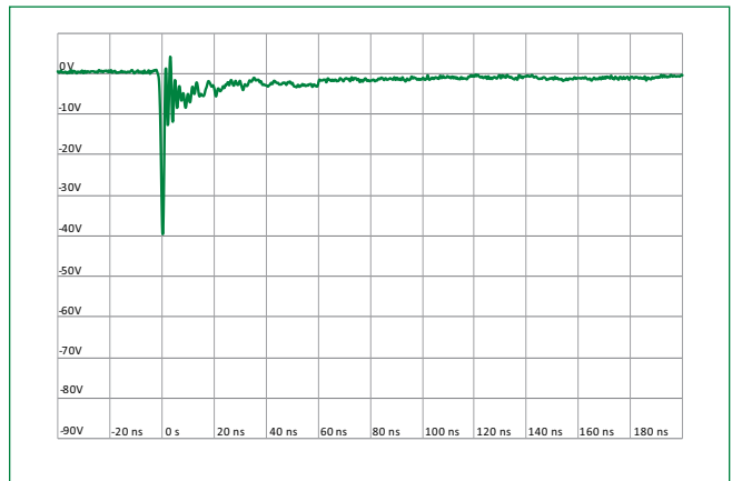
IEC 61000-4-2 -8 kV Contact ESD Clamping Voltage
