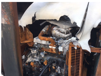
Mobile generator destroyed by arc-flash.
