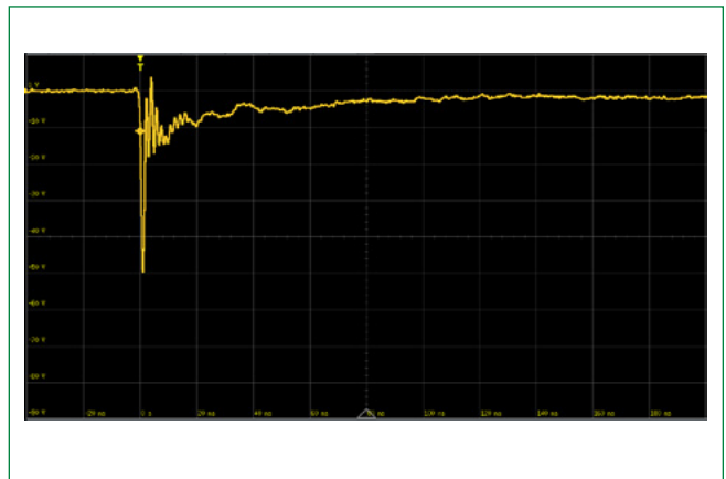
IEC 61000-4-2 -8 kV Contact ESD Clamping Voltage
