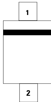
Cathode polarity for unidirectional only
