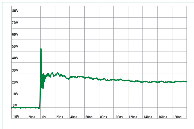
IEC 61000-4-2 +8 kV Contact ESD Clamping Voltage
