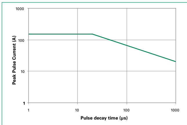
Figure 1: Non-repetitive Peak Pulse Current vs. Pulse Time
