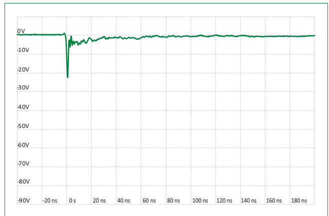
IEC 61000-4-2 -8 kV Contact ESD Clamping Voltage
