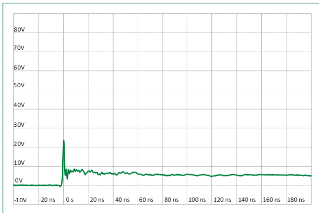
IEC 61000-4-2 +8 kV Contact ESD Clamping Voltage
