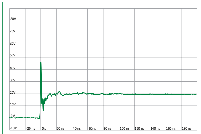
IEC 61000-4-2 +8 kV Contact ESD Clamping Voltage
