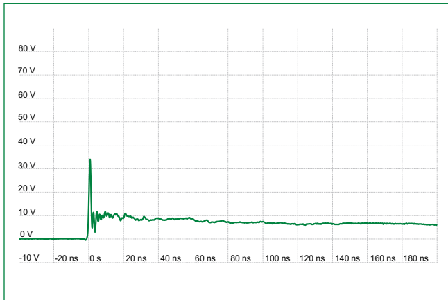
IEC 61000-4-2 +8 kV Contact ESD Clamping Voltage
