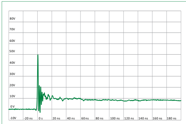
IEC 61000-4-2 +8 kV Contact ESD Clamping Voltage
