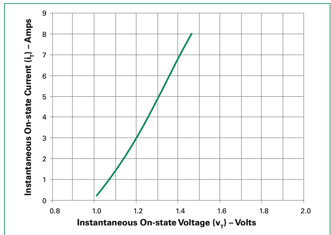
Figure 2: On-state Current vs. On-state Voltage (Typical)
