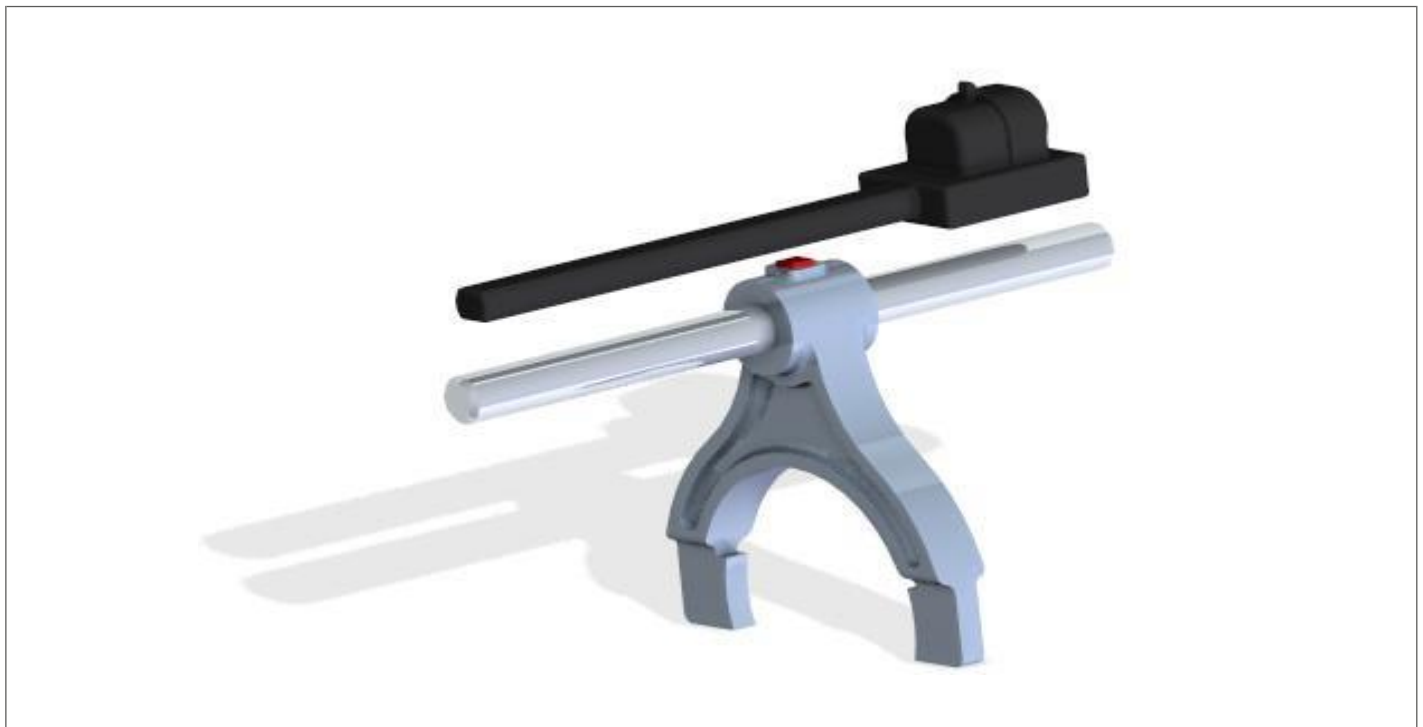
Figure 7: Fork Position measurement using PWG sensor
