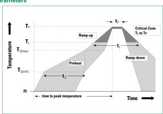
1. Tolerance for peak profile temperature  $\left(T_{p}\right)$  is defined as a supplier minimum and a user maximum.
