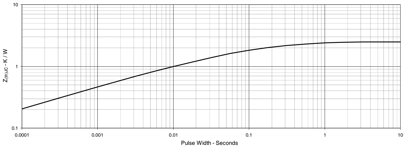
Fig. 11. Maximum Transient Thermal Impedance
