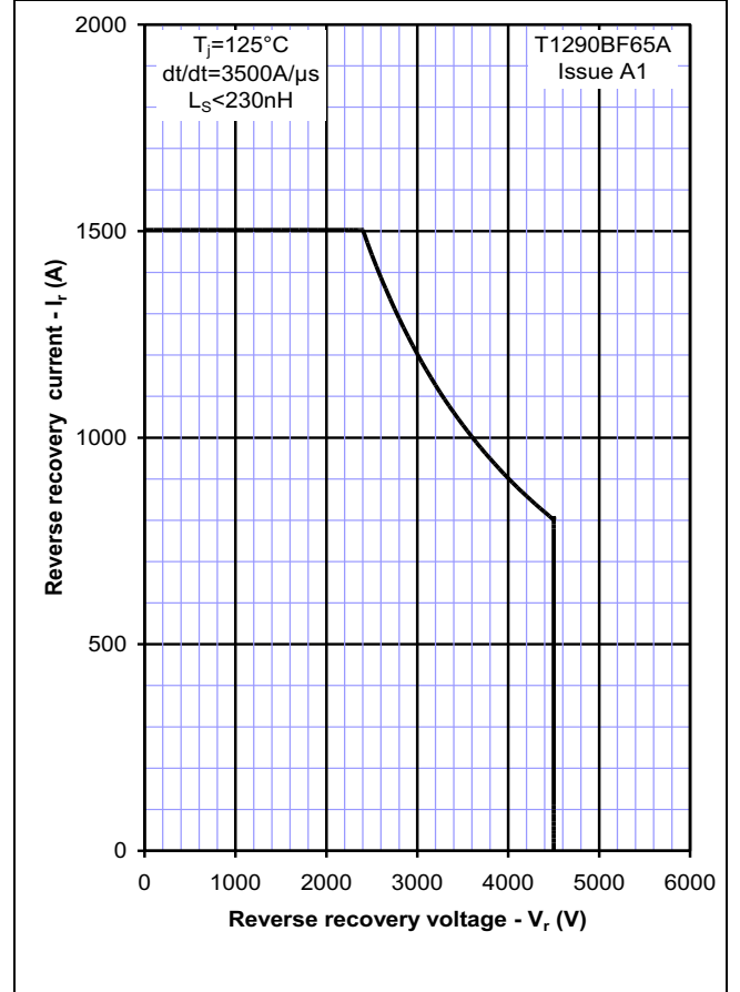
Figure 6 – Safe operating area (Diode)
