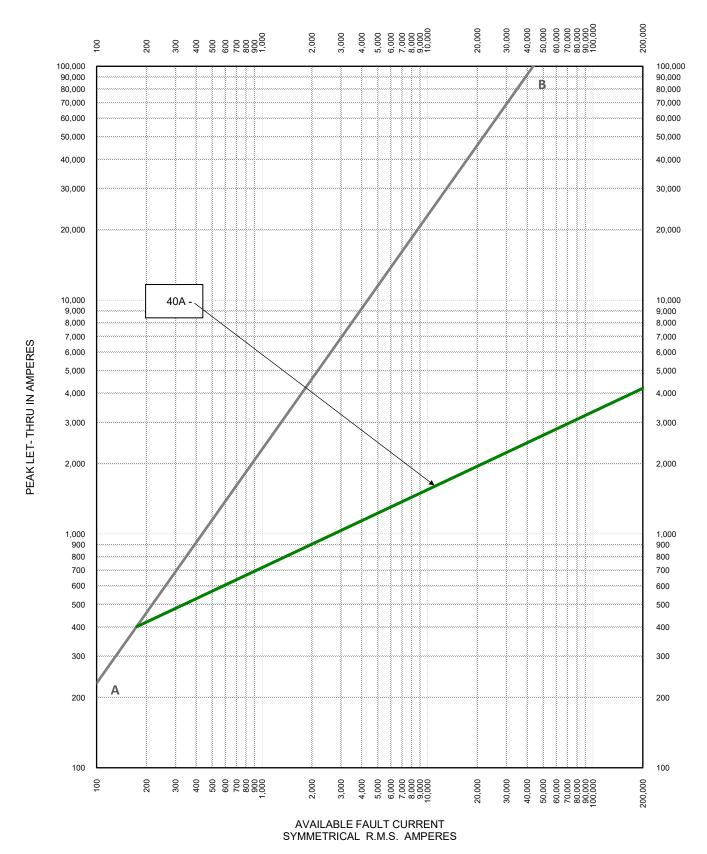
TIME CONSTANT/POWER FACTOR: FUSE CATALOG NUMBER: TEST VOLTAGE: L60QS 40 A BASIS FOR DATA: AB = 15% Power Factor DRAWN BY: LLL LITTELFUSE, INC. DATE: 02/29/2024 CHICAGO, IL. USA REVISION: DRAWING NO.: SHEET 2 OF 2 PEAK LET-THRU CHARACTERISTIC CURVES
