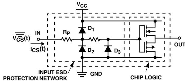
FIGURE 9. TYPICAL CMOS IC INPUT PROTECTION CIRCUIT
