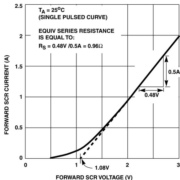
FIGURE 7. SCR FORWARD CURRENT vs VOLTAGE CHARACTERISTICS
