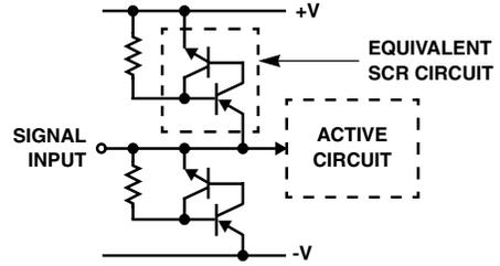
FIGURE 4. PROTECTION CELLS OF THE SP720 SCR ARRAY
