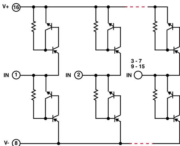
FIGURE 6. EQUIVALENT CIRCUIT DIAGRAM OF THE SP720
